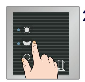
Close the door and press one of the program buttons to start the drying. For energy-efficient drying, run the machine fully loaded, and do not open the doors of the drying cabinet during the drying process.
